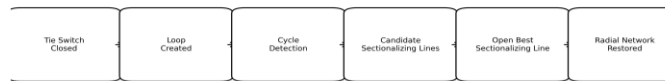
Figure 3. Radiality-preserving restoration repair mechanism. Source: Authors' algorithmic design implemented in the simulation notebook.
