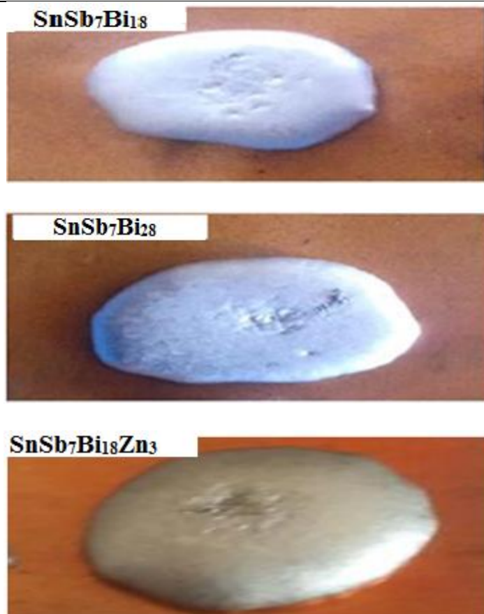
Figure 3: spreading of used alloys on pure Cu substrate in air
